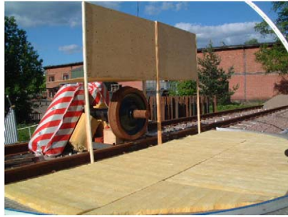
Fig. 4. The set-up for measuring the shielding effect of car-body on vertical directivity [6].
